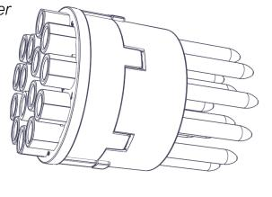
Insert the crimped socket contacts into the equipped contact holder and snap into place.
