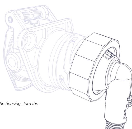
Slide the bayonet ring and end cap onto the housing. Turn the bayonet ring onto the housing.
