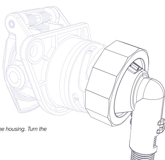
Slide the bayonet ring and end cap onto the housing. Turn the bayonet ring onto the housing.
