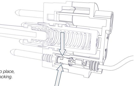
After the socket contacts have snapped into place, please check the correct assignment and locking.
