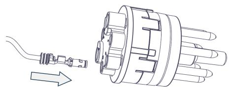
Insert the crimped socket contacts into the equipped contact holder and snap into place.
